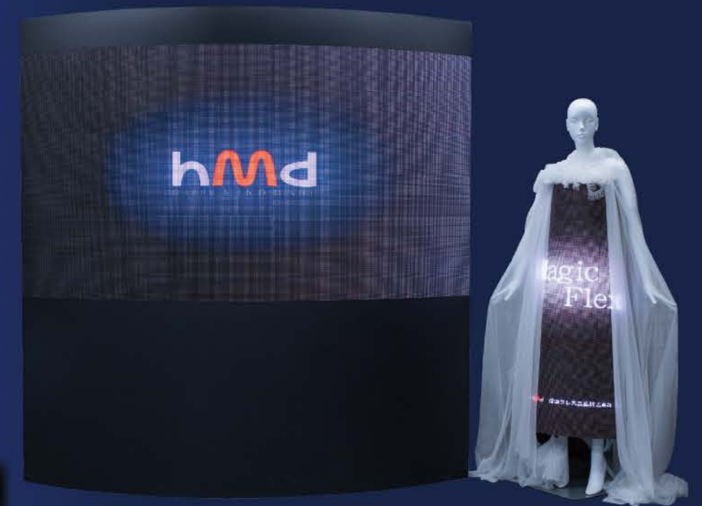
MagixFlex P4 1 Piece Spec 256mm × 192mm 64dots × 48dots RGB Full Color
